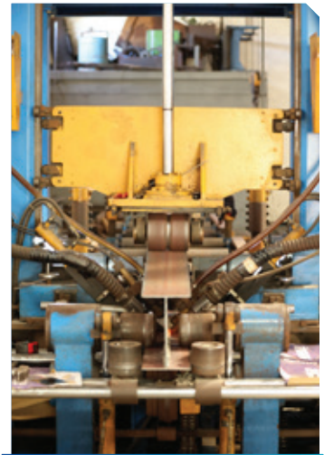
3 in 1 Machine (Beams Assembly, Welding & Straightening)
